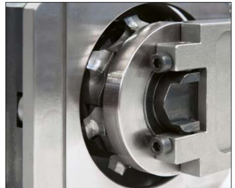
flexTrim am Formfräsaggregat
