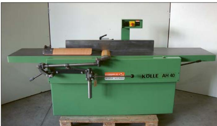
Abrichtobelmaschine Kölle AH 40
